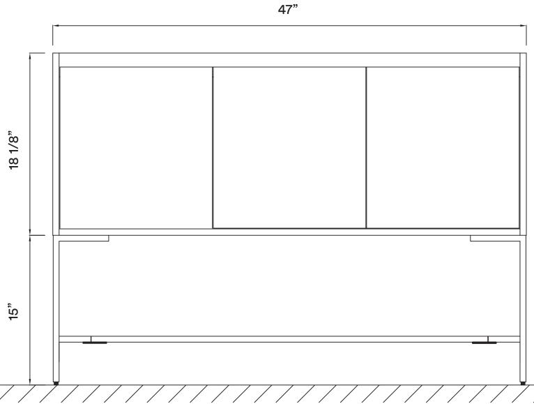
ATTENTION! Dimensions may vary by up to 3/8". It is highly recommended to pull all dimensions of actual model for installation and measuring purposes.
